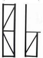
The welded steel end frames have two rows of slots.
