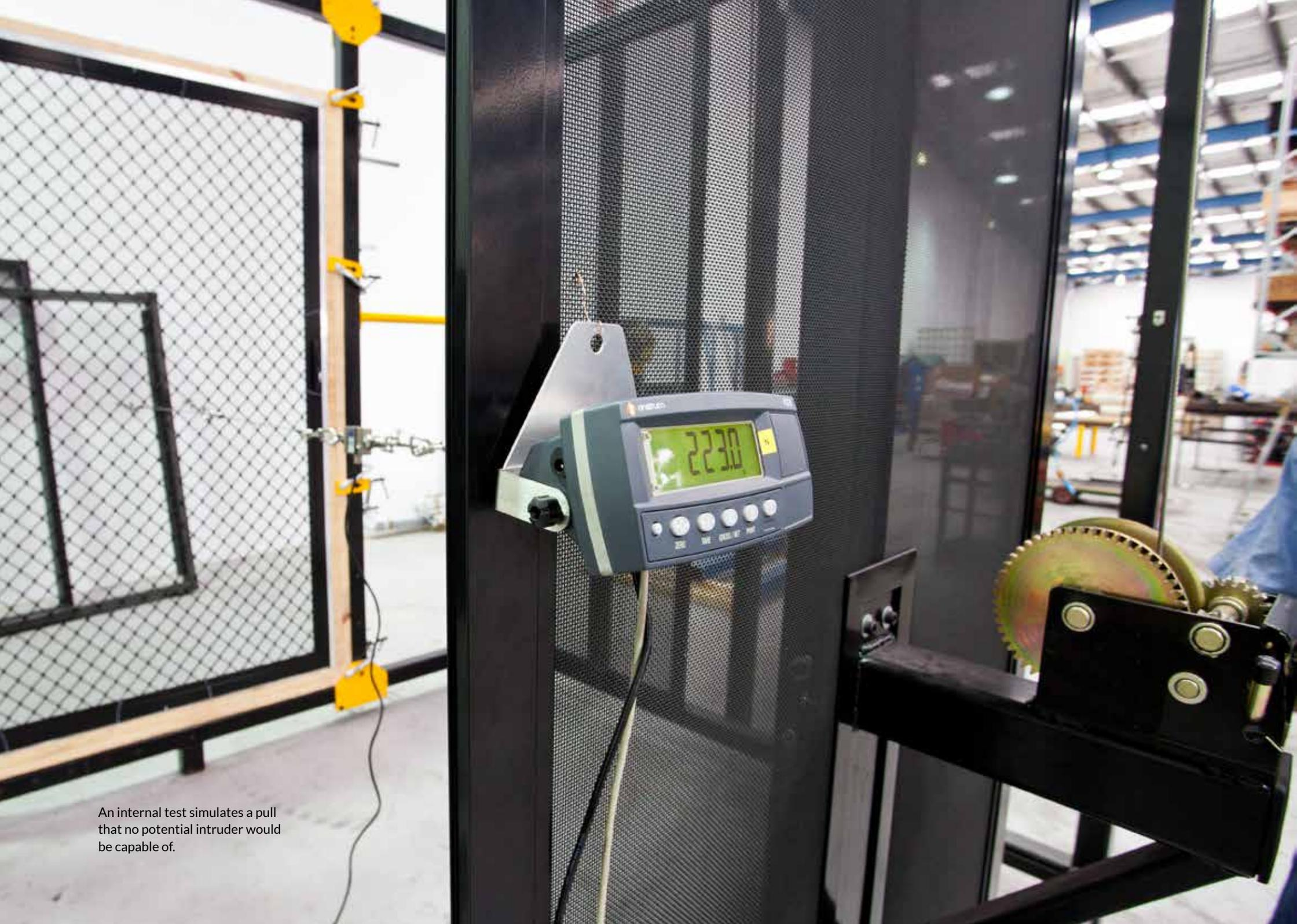
An internal test simulates a pull that no potential intruder would be capable of.
