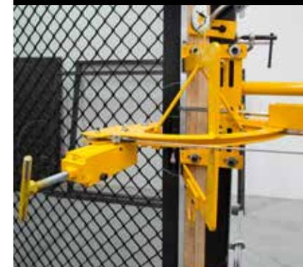
This internal test simulates an attack with a screwdriver.
